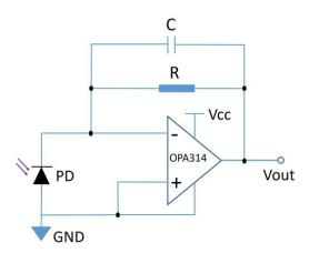
$$\begin{split} &V_{out}(V) = I_{ph}(A) \times R \; (\Omega) \\ &I_{ph}(A) = R_{\lambda}(A/W) \times A \; (cm^2) \times P \; (W/cm^2) \\ &\text{where A is chip area, P is incident UV power density} \\ &\text{and } R_{\lambda} \; \text{is responsivity at specific wavelength.} \end{split}$$
