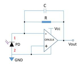
$V_{out}(V) = I_{ph}(A) \times R(\Omega)$
