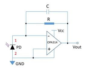
$V_{out}(V) = I_{ph}(A) \times R(\Omega)$  $I_{ph}(A) = R_{\lambda}(A/W) \times A(cm^2) \times P(W/cm^2)$ where A is chip area, P is incident UV power density and R\_{\lambda} is responsivity at specific wavelength.
