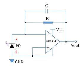
$V_{out}(V) = I_{ph}(A) \times R(\Omega)$
