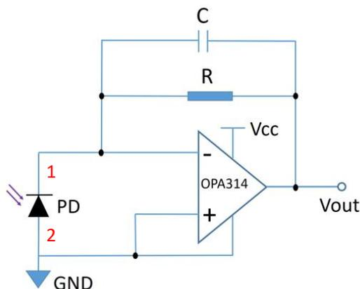
$$V_{out} (V) = I_{ph} (A) \times R (\Omega)$$
