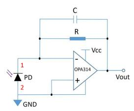
$$\begin{split} &V_{out}(V) = I_{ph}\left(A\right) \times R \; (\Omega) \\ &I_{ph}\left(A\right) = R_{\lambda}(A/W) \times A \; (cm^2) \times P \; (W/cm^2) \\ &\text{where A is chip area, P is incident UV power density} \\ &\text{and } R_{\lambda} \; \text{is responsivity at specific wavelength.} \end{split}$$
