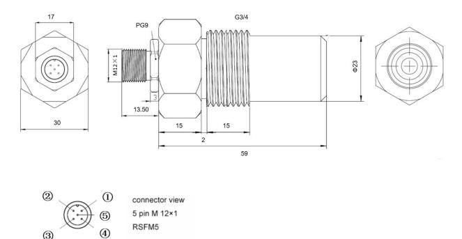
5-pin analog plug: pin 1=V<sub>cc</sub>, pin 2=null, pin 3=I<sub>out</sub> / V<sub>out</sub>, pin 4=GND / null, pin 5=null
